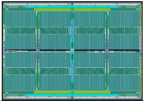
**Figure 2. Gemini chip photo.** Rather than combining a large processor and a memory on one die, the design interleaves more than 2 million tiny processing units among 48 million memory cells, creating a highly regular structure.
