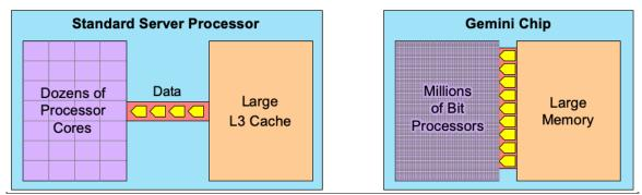
**Figure 1. Breaking the memory bottleneck.** Traditional processors (left) struggle with large datasets due to the narrow connection with the large on-chip memory. Gemini features millions of cores that can all access memory at once, allowing a much greater flow of data.
